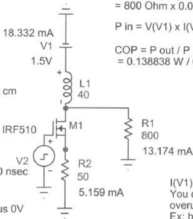
$$P_{out} = R(R1) \times I(R1) \times I(R1) = 800 \text{ Ohm} \times 0.013174\text{A} \times 0.013174\text{A} = 0.027498 \text{ W}$$
