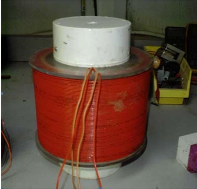
Norm's Large MRA wound on 4" ID ferrite magnets to light 8 foot fluorescent tubes with an audio amp input
