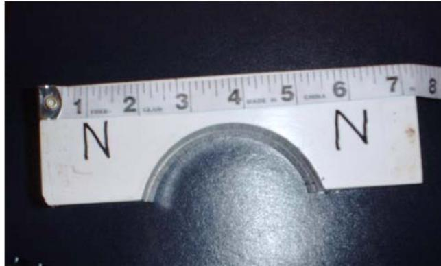
A Barium ferrite magnet taken from an old IBM main frame hard drive
