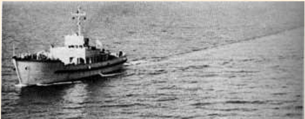
**The *HMS Repulse* sweeping the waterways using streamed cables.**
