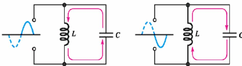
(a) The coil deenergizes as the capacitor charges.
