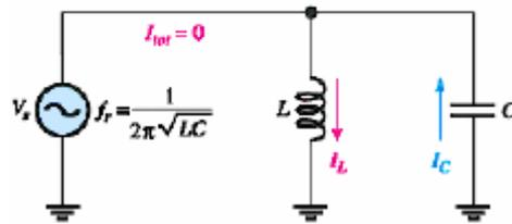
(a) Parallel circuit at resonance ( $X_C = X_L, Z = \infty$ )
