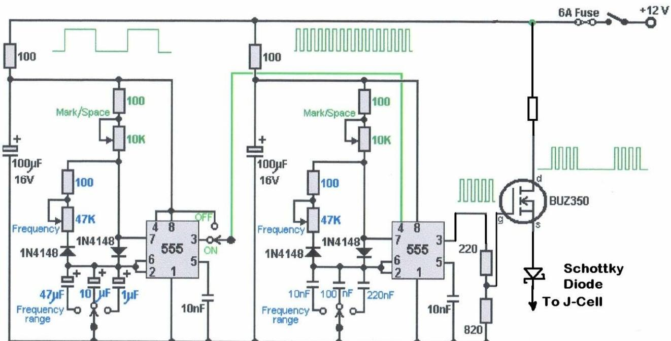
2. Component **28** on Gray's circuit is a diode. Preferably use a Schottky diode for fast switching. This diode is absolutely essential, as it ensures that no negative pulses or reverse pulses are allowed to traverse the "secret path".
