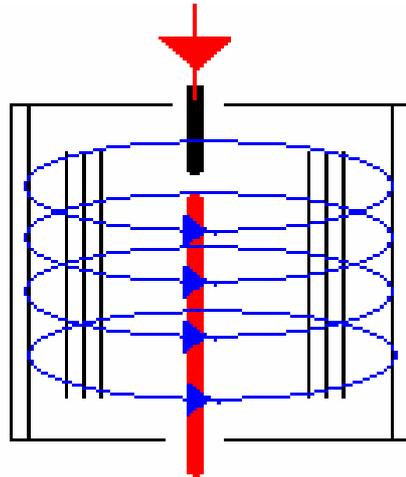
Utilizing the principle that the inductance produced by one turn of wire about a core of permeability  $n$  is electrically equivalent to a coil of the same cross section wound with  $n$  turns of wire, the central conductor of the J-cell forms a single turn induction coil with water functioning as its magnetic core.
