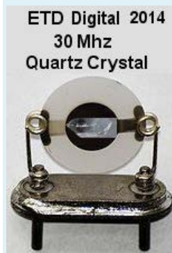
- Larger 30MHZ Quartz Crystal Core
