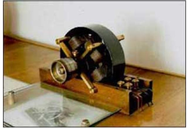
One of Tesla's 2 phase induction motors. When linked to his polyphase method of generating and transmitting electricity, this motor became the foundation stone on which the modern electrical power industry is built.
