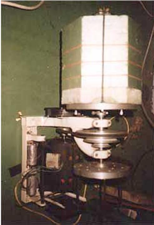
**This is a picture of a pressing apparatus used in the sintering process. The different ring-roller elements are heated and pushed together under several tonnes per square inch.**
